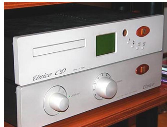
Back to today's stereo integrated. With 2-100,000Hz bandwidth, 9.5dB of feedback and the firm's "improved dynamic Class 'A' symmetrical stage with complementary power MOSFET pair" architecture, the Unico consumes 340 watts at full boogie, weighs a stolid 35 lbs but only measures 17" x 13.5" x 3.75" WxDxH.
