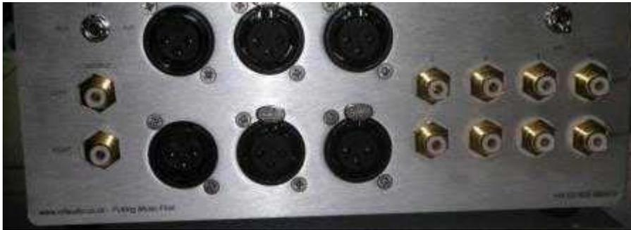
*Above: The rear panel of the MF amp with single-ended and balanced connections*
