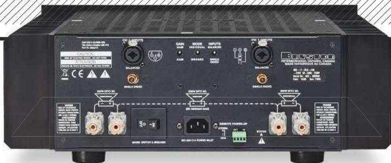
ABOVE: Single-ended (RCA) and balanced ins (combined XLR and 0.25in jack sockets) are joined by 1V and 2V input sensitivity options, a bridged output option, remote or local input switching and a single set of unswitched 4mm speaker binding posts
